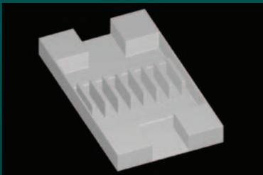
With FAVOR™, a simple structured grid results in a well-resolved geometry. *FLOW-3D* can be used to accurately and efficiently simulate flow in complex microchannels, chambers and other devices.
