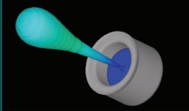
*FLOW-3D's* TruVOF technique allows for accurate representation of moving liquid fronts.
