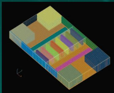
With Multi-Block meshing capabilities in *FLOW-3D*, you can easily and efficiently capture complex geometries and apply varying degrees of resolution for sharper modeling.
