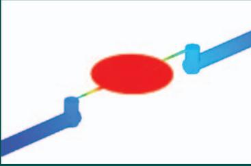
An instantaneous pressure distribution of the piezoelectric pump system, which is calculated using the elastic membrane model.
