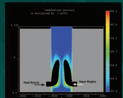
**FLOW-3D's** interface and free-surface tracking technology allows users to simulate multi-phase flows quickly and easily without complicated meshing procedures. **FLOW-3D** can also simulate evaporation and condensation at these surfaces.
