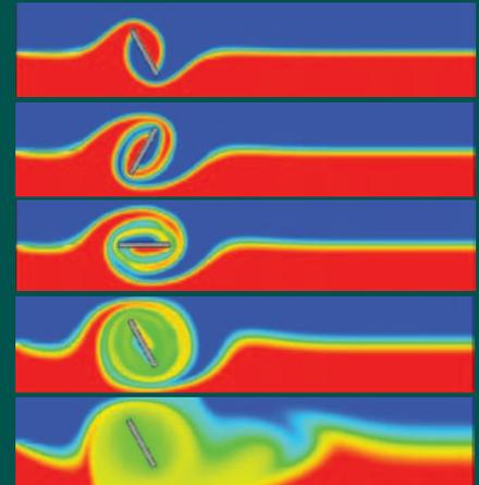
Microscale fluid mixing is crucial and challenging for microfluidic system applications. Active and passive micromixers aim to achieve maximum mixing efficiency in the least amount of distance and time. **FLOW-3D** can model molecular and eddy diffusion for different complex mixer geometries to achieve efficient and optimal design.
