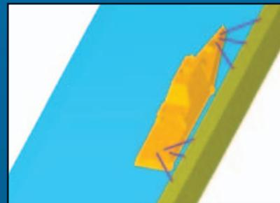
Simulation of a moored ship using the strings & ropes capability in **FLOW-3D**'s GMO model.
