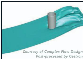
**Wave Impact:** Load predictions on marine structures such as oil production platforms in random storm waves are critical. Physical mechanisms leading to water on deck and bow flare slamming, and the resulting responses, must also be analyzed. **FLOW-3D** provides
