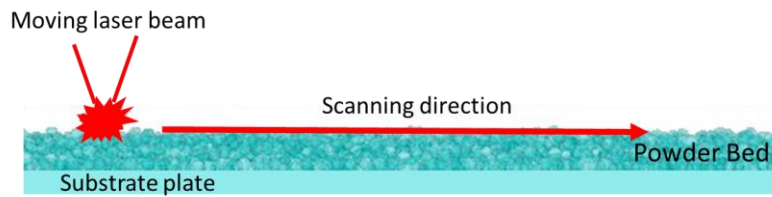
Figure 1. The schematic of the powder bed and scanning direction of moving laser beam
