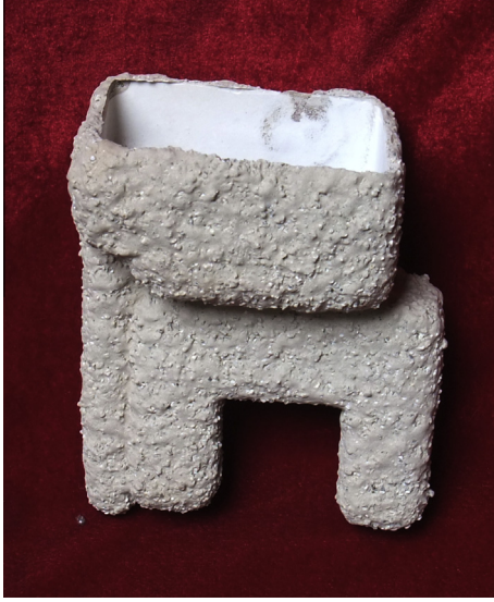
Fig. 3. Ceramic shell (including pouring basin) after burning step.
