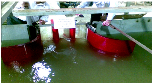
Figure 2 Sketch of scaled laboratory model of the Balaroud guide wall dam.
